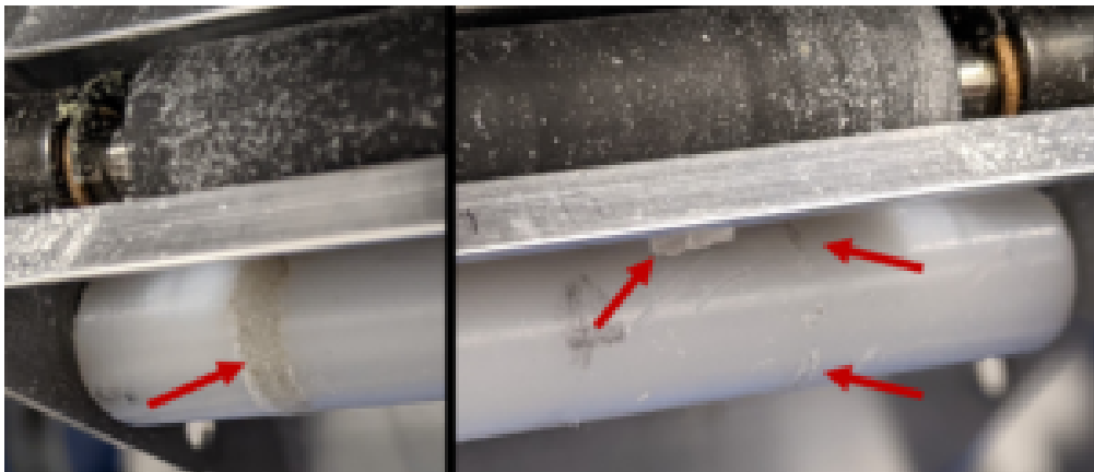
ABOVE: Paper fiber build-up on platen roller. Adhesive build-up and label pieces (red arrows) on pinch roller.
